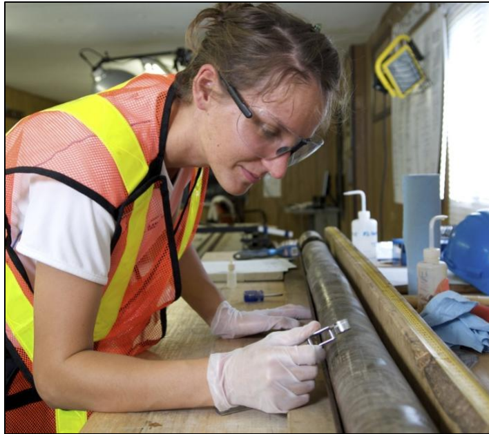
Researcher studies samples of limestone rock drilled from one of eight boreholes around DGR site.
